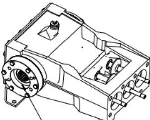
ASSEMBLE BEARING HOUSING
